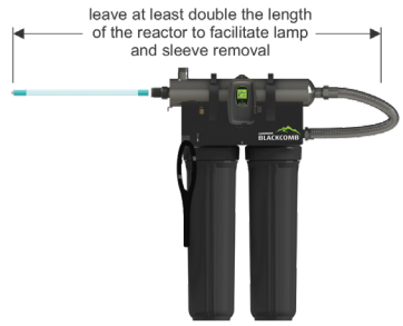
Figure 3. Lamp Removal Spacing
