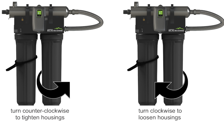
Figure 5. Cartridge Removal
